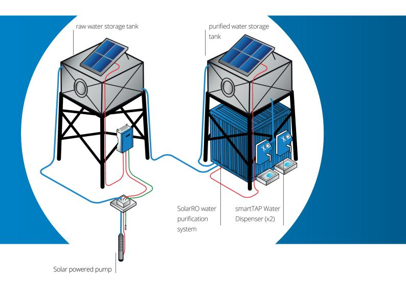
Two **smartTAP Water Dispensers** have been integrated into the containerized water purification system, providing an easy, secure and affordable solution for dispensing water. The smartTAP dispenses clean water using a simple to operate NFC tag.
