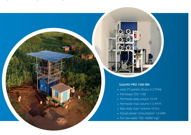
The SolarRO water purification system makes clean drinking water without chemicals and emissions, directly from seawater, impure lakes and rivers, or saline boreholes. The unit has been certified as yielding excellent quality drinking water according to the World Health Organization (WHO) standards.
